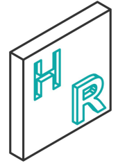
Emboss & Engrave Horizontal >0.9mm wide, <0.9mm deep
